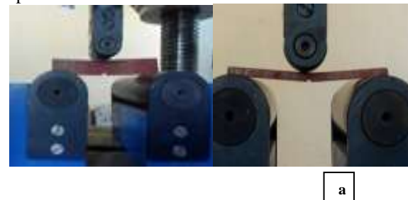
Fig. 6 Experimental set-up for flexural test a) Edge notch b) Width notch
